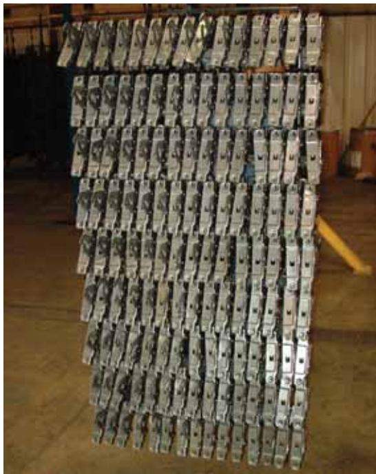
Maximizing the load bar density while reducing and eliminating rejects is one key to an e-coater's success.
